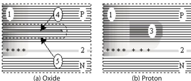
Figure 11. VCSEL current confinement structures.
