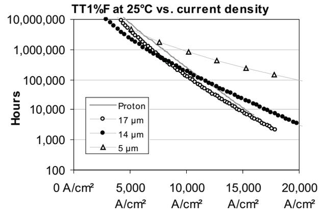
Figure 6. Reliability as a function of current density. Despite having lowest reliability at typical operating levels, smallest device is actually disproportionately more reliable in this physically fundamental sense.
