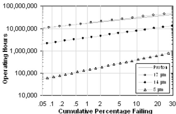
Figure 2. Comparative reliability of different designs at 25°C and nominal operating currents (10, 8, 6.5, and 3.5 mA for Proton, 17 μm, 14 μm, and 5 μm respectively).
