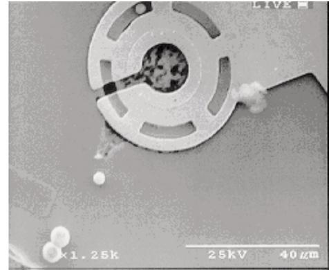
Figure 10. If only they were all so easy to diagnose! VCSEL subjected to EOS which explosively melted material in the active region and under the contact, depositing ejecta some distance away.
