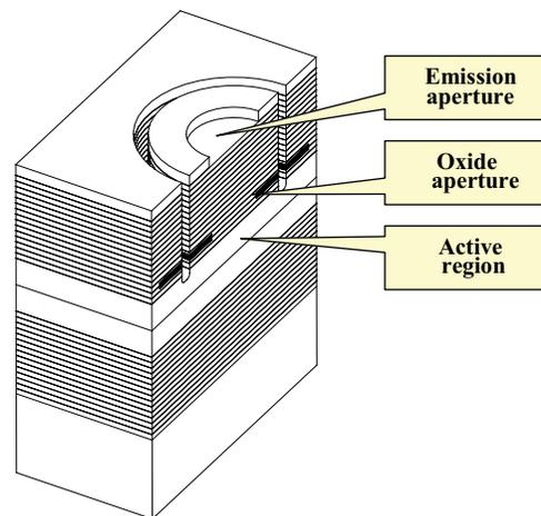
Figure 1. Schematic cross-sectional view of an oxide-isolated VCSEL.
