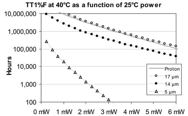
Figure 5. Reliability as a function of emitted power. The reliability is calculated at 40°C, but based on the current necessary to achieve the stated power at 25°C. Note the inversion of which device is most reliable compared to the previous figures.
