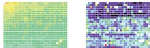
Figure 17. Comparison of forward voltage measured on-wafer, before any burn-in (left), and in TO-components after burn-in (right). Both the average level and the small-scale variation change.
