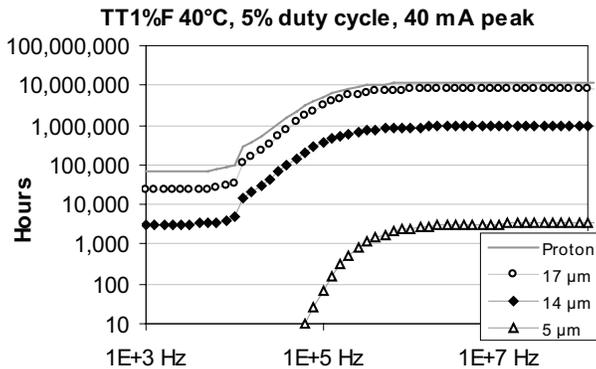
Figure 8. Calendar reliability as a function of repetition frequency for pulsed operation at a fixed duty cycle and peak current. For the same average power dissipation, reliability can vary over three orders of magnitude.
