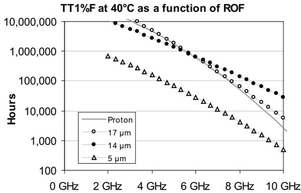
Figure 7. Reliability as a function of Relaxation Oscillation Frequency. This is a fundamental measure of likely modulation performance; it depends on the square root of the ratio of stimulated current to threshold current. The medium-sized oxide is most reliable by this metric.
