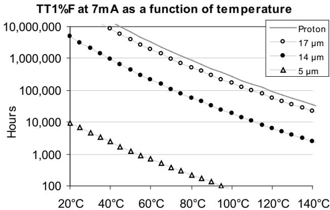
Figure 3. Reliability as a function of ambient temperature at a fixed current.
