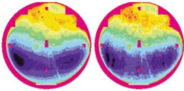
Figure 14. Full wafer maps of threshold current, for the same wafer as in Figure 13. As in the case of forward voltage, short-range variation increases.
