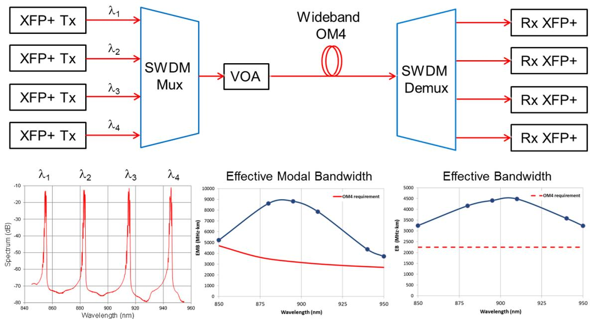
**Fig. 1:** Experimental setup, including measured SWDM spectrum, and wideband OM4 measured EMB and EB (SBW=0.4nm).
