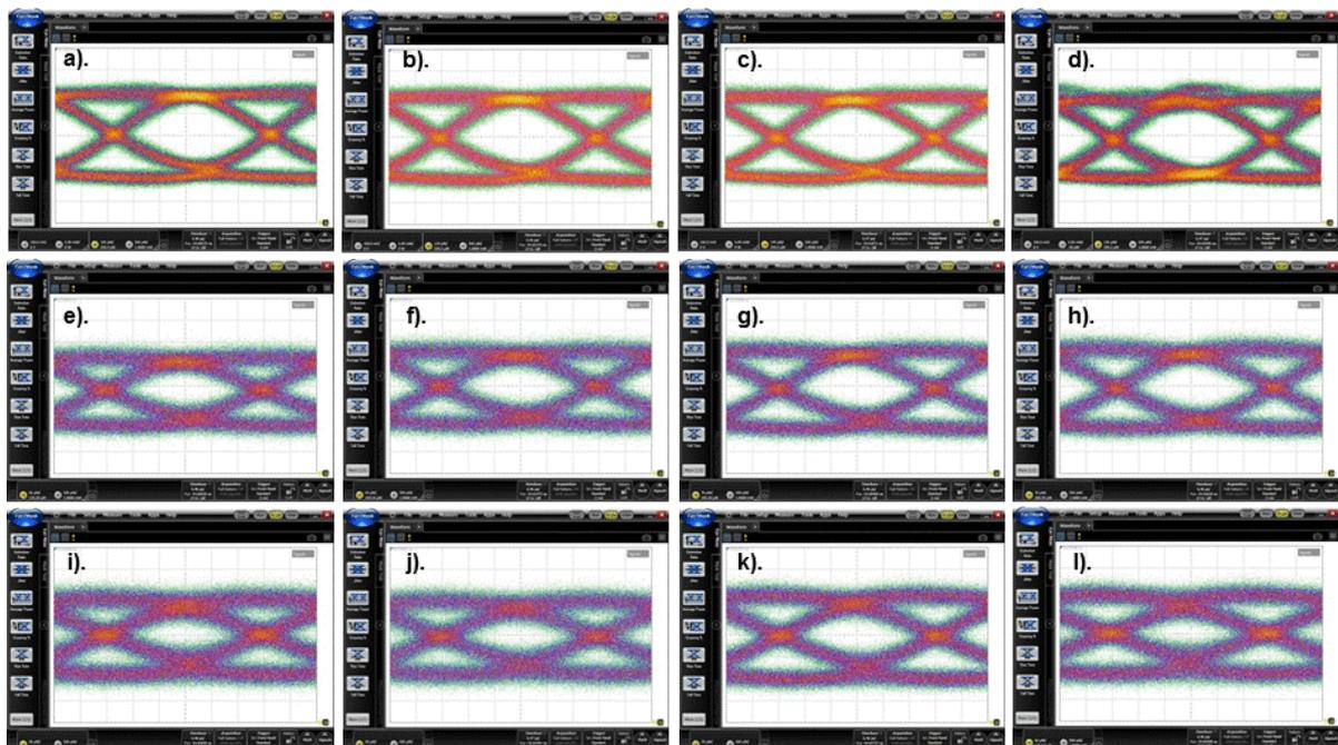
**Fig. 2:** Measured optical eye diagrams for a)-d). transmitter eyes, e).-h). received eyes for 200m, and i).-l). received eyes for 300m; note leftmost column corresponds to 855nm channel, with increasing wavelength to 945nm for rightmost column.
