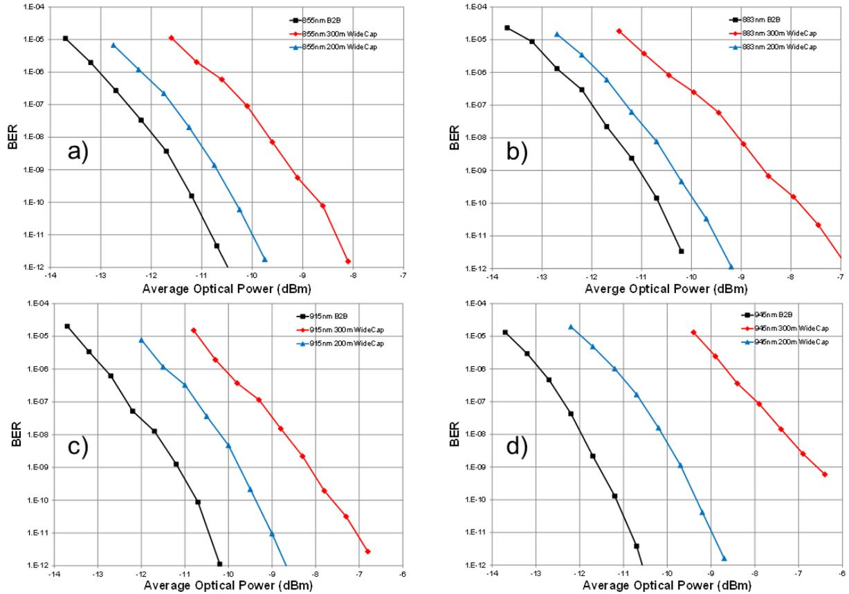
**Fig. 3:** Measured BER B2B (black), 200m (blue), and 300m (red) for a). 855nm, b). 883nm, c). 915nm, and d). 945nm channels.
