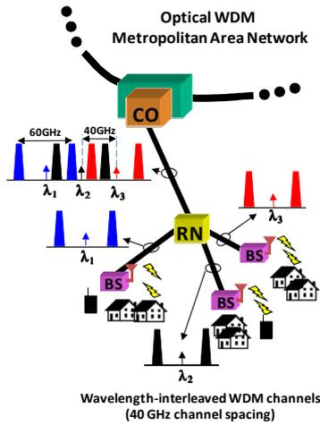
Fig. 12 60 GHz WDM fiber-wireless system incorporating wavelength interleaved scheme to improve spectral usage
