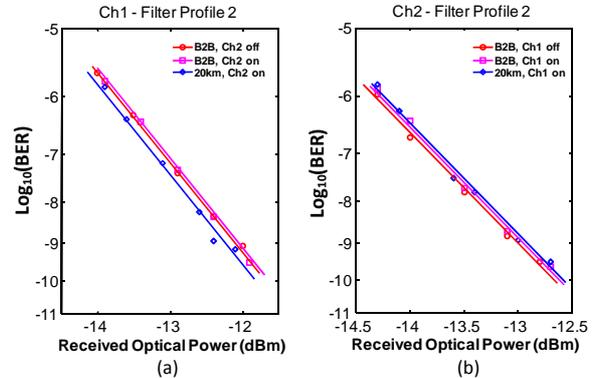
Fig. 8 Measured BER curves (a) Ch1 and (b) Ch2 with RN programmed with filter profile 2
