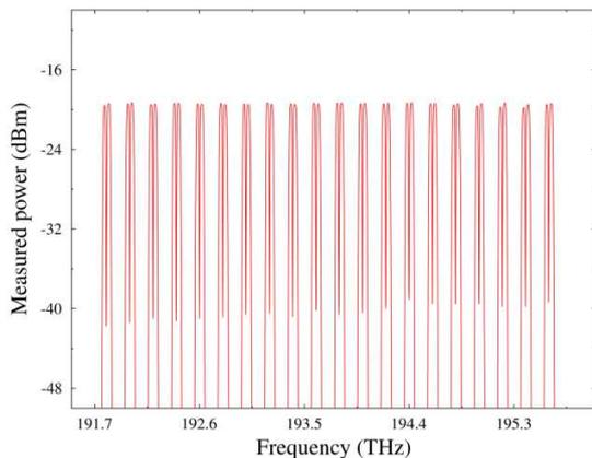
Fig. 18 Gain flattening at the RN after a channel upgrade from 25 to 40 channels.
