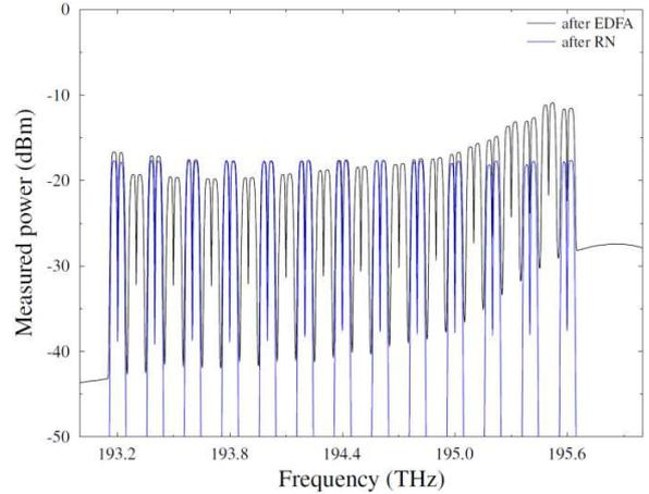
Fig. 16 Gain flattening and demultiplexing 60 GHz fiber-wireless channels in the POP-based RN.
