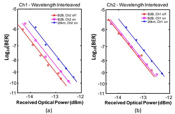
Fig. 14 Measured BER curves for (a) Ch1 and (b) Ch2 for wavelength interleaved channel allocation
