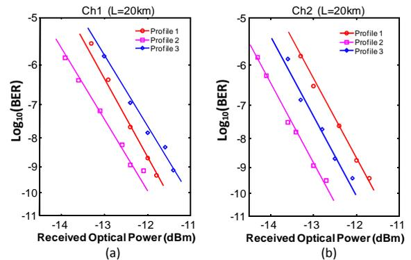
Fig. 11 Comparison of BER curves for all filter profiles for transmission over 20 km of SMF for (a) Ch1 and (b) Ch2
