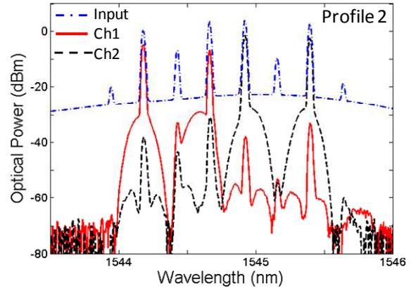
Fig. 7 Measured optical spectra before and after RN for filter profile 2
