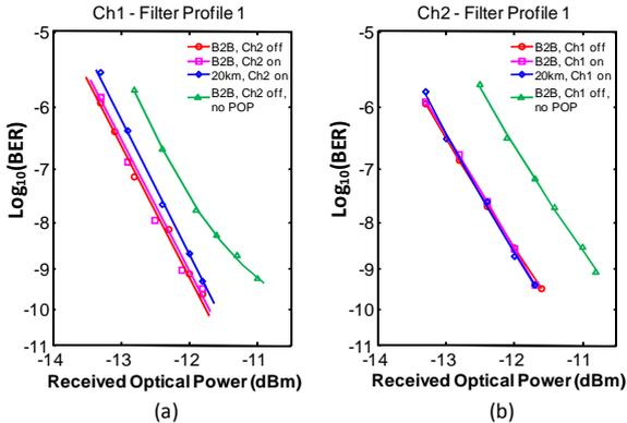
Fig. 6 Measured BER curves (a) Ch1 and (b) Ch2 with RN programmed with filter profile 1
