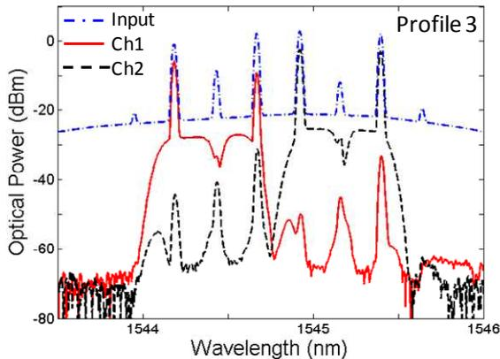
Fig. 9 Measured optical spectra before and after RN for filter profile 3
