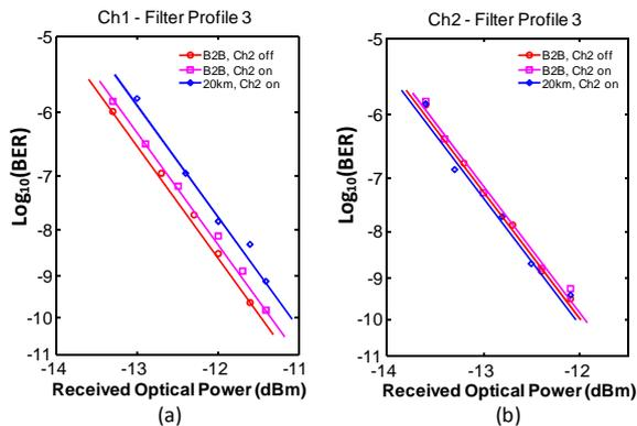
Fig. 10 Measured BER curves (a) Ch1 and (b) Ch2 with RN programmed with filter profile 3
