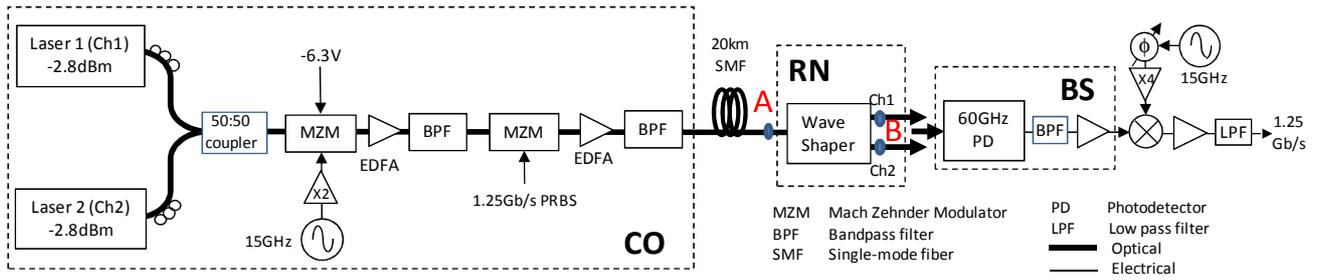
Fig. 4 Experimental setup for 60 GHz fiber-wireless link characterization using programmable optical processor (POP) in RN
