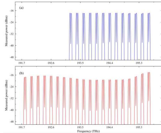
Fig. 17 The impact of channel plan upgrades on the demultiplexed output of the POP-based RN. Initially, (a) channels are well balanced, but (b) poorly balanced upon the addition of 15 more channels.
