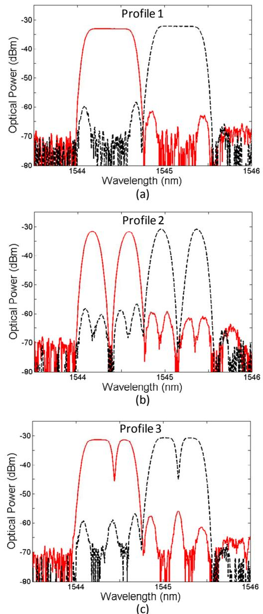
Fig. 3 Filter profiles to be investigated for 60 GHz WDM fiber-wireless links: (a) flattop, (b) flattop with stopband, and (c) flattop with phase notch.
