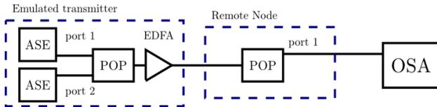
Fig. 15 Experimental setup to demonstrate reconfigurability and dynamic functionality of the POP-based RN.
