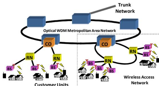
Fig. 1 WDM fiber-wireless network architecture
