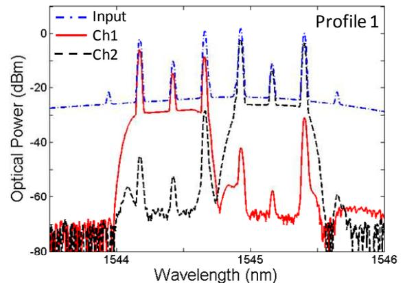
Fig. 5 Measured optical spectra before and after RN for filter profile 1
