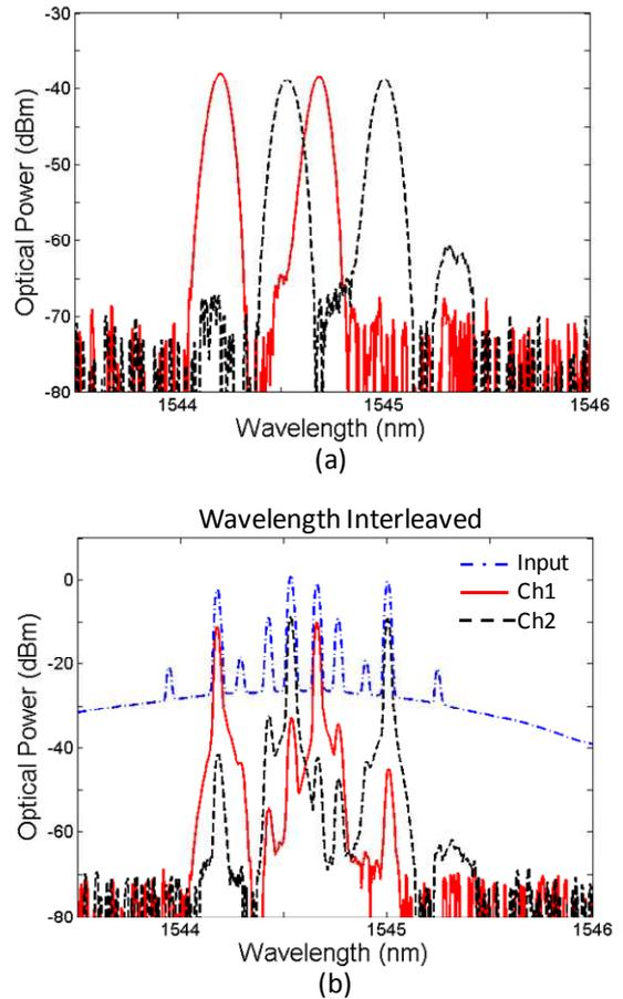
Fig. 13 (a) Measured filter profile for demultiplexing interleaved channels (b) Measured optical spectra before and after RN for wavelength interleaved 60 GHz fiber-wireless link
