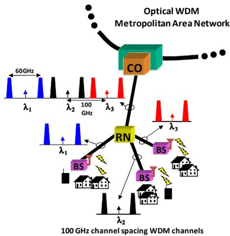
Fig. 2 60 GHz WDM fiber-wireless system with 100 GHz channel spacing
