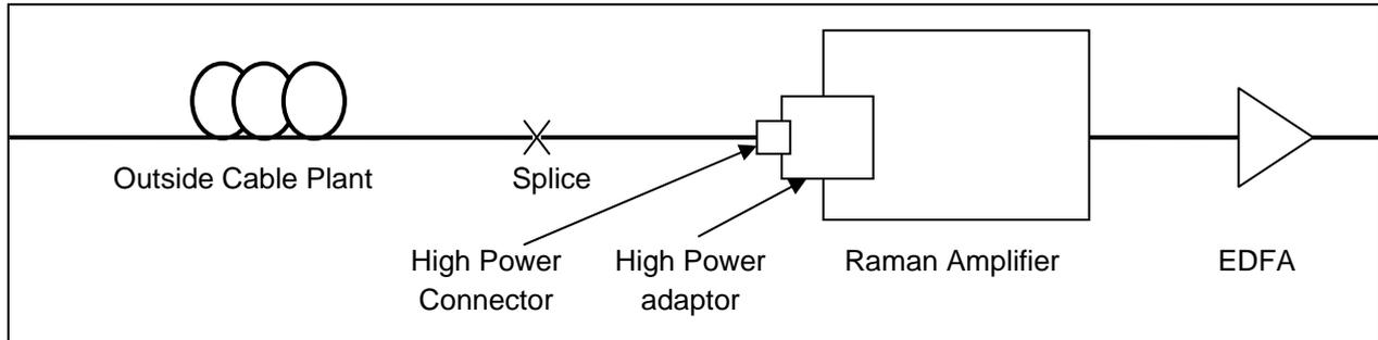
Figure 3: Connecting the Raman Amplifier to the outside cable plant
