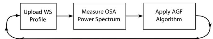
Figure 2: Illustrates the algorithm feedback loop used in the AGF system.
