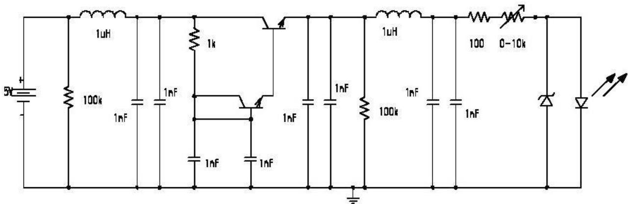
Figure 1. Schematic for a slow starting constant current source to drive a VCSEL.
