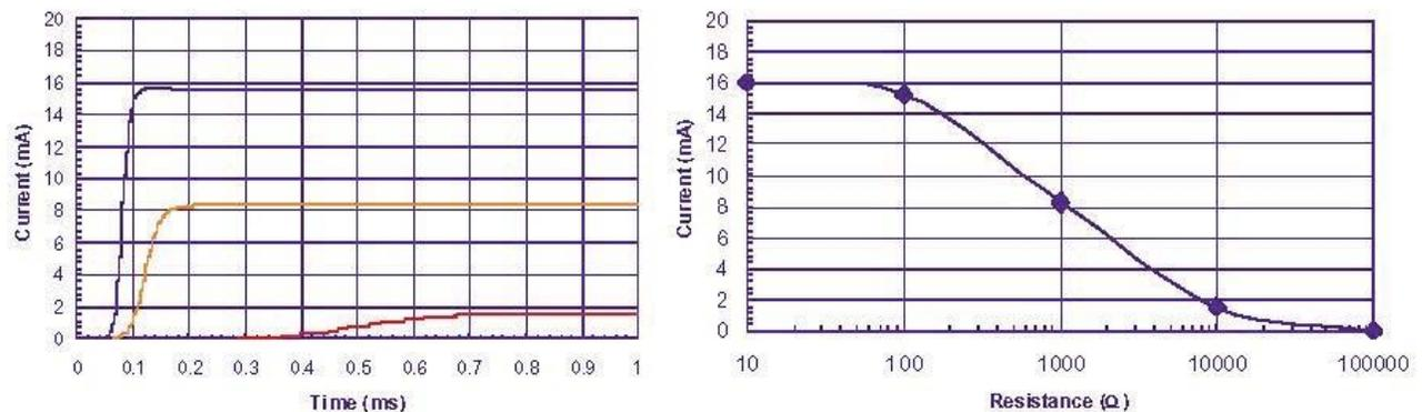
Figure 4 (a) Turn on transient of the APC circuit of figure 3 for various values of the potentiometer, and (b) the final current value as a function of the control resistance
