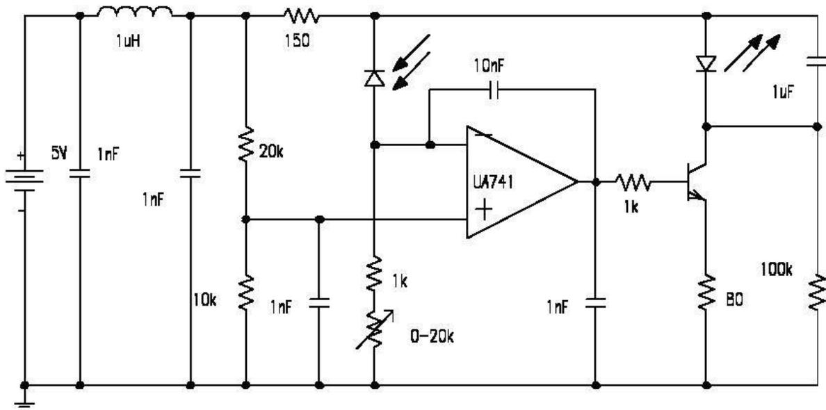
Figure 3. Schematic for an Average Power Control Circuit
