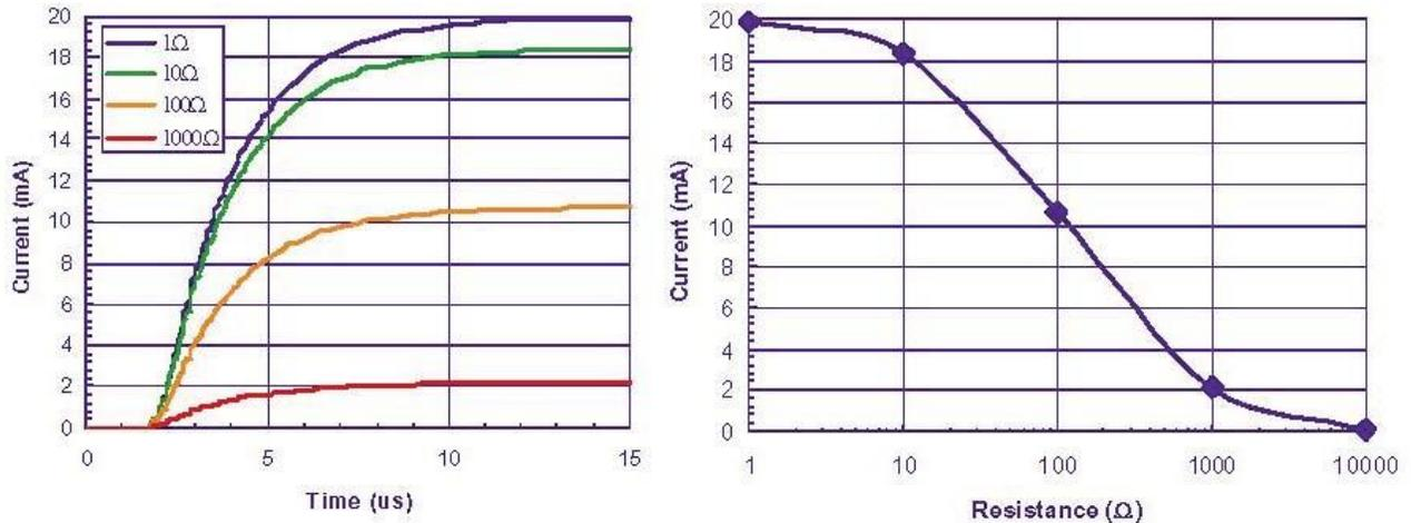
Figure 2 (a) Turn response of the circuit in Figure 1 for several potentiometer values.
