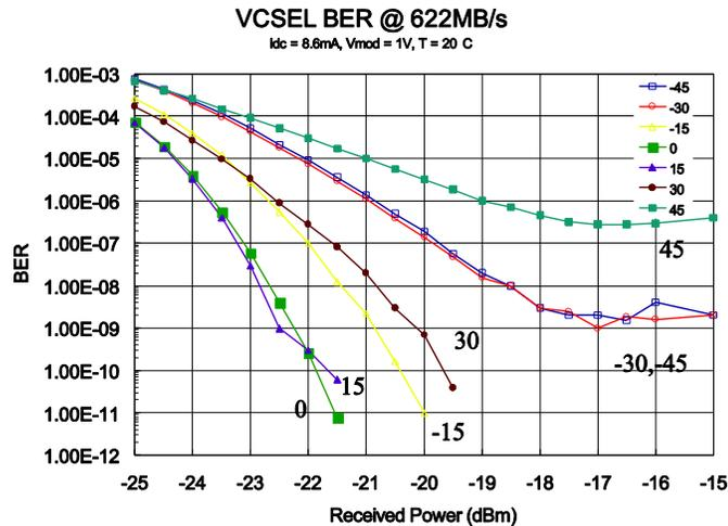
Figure 11. Measured BER with polarization selective coupling loss.
