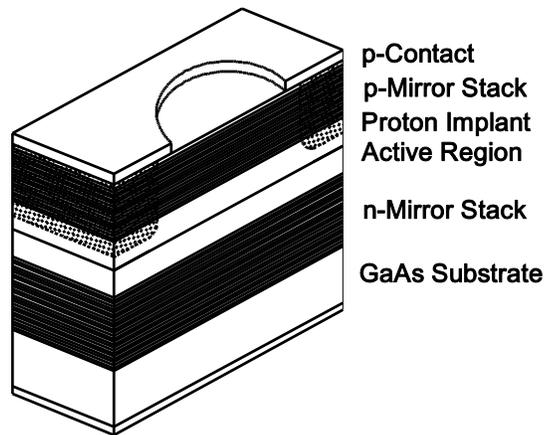
Figure 1. Schematic of a VCSEL.
