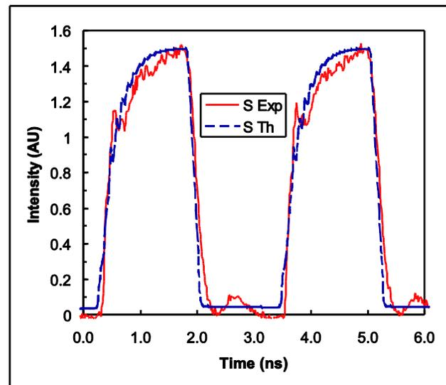
Figure 10. Output from the VCSEL with the polarizer at -45 degrees.
