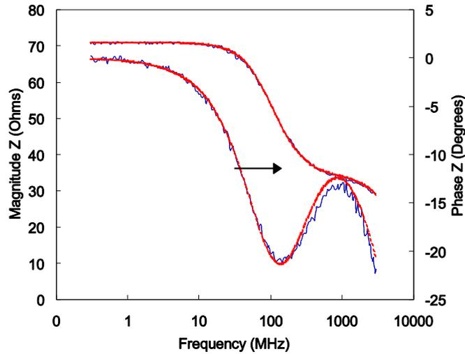
Figure 4. Measured and calculated VCSEL impedance
