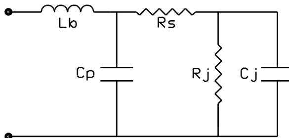
Figure 3 VCSEL Equivalent circuit
