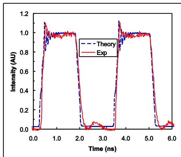
Figure 8. Output from the VCSEL with the polarizer at 0 degrees.
