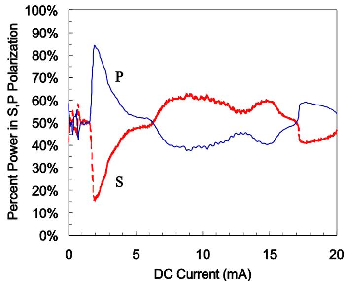
Figure 7 Percent power in the S and P modes of a VCSEL.
