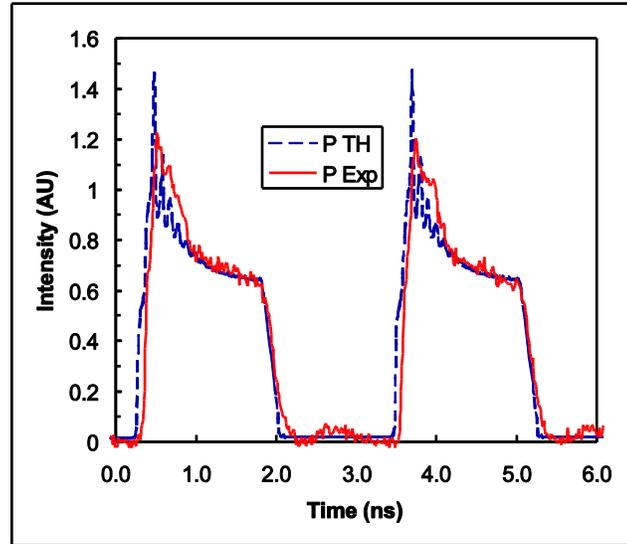
Figure 9. Output from the VCSEL with the polarizer at +45 degrees.
