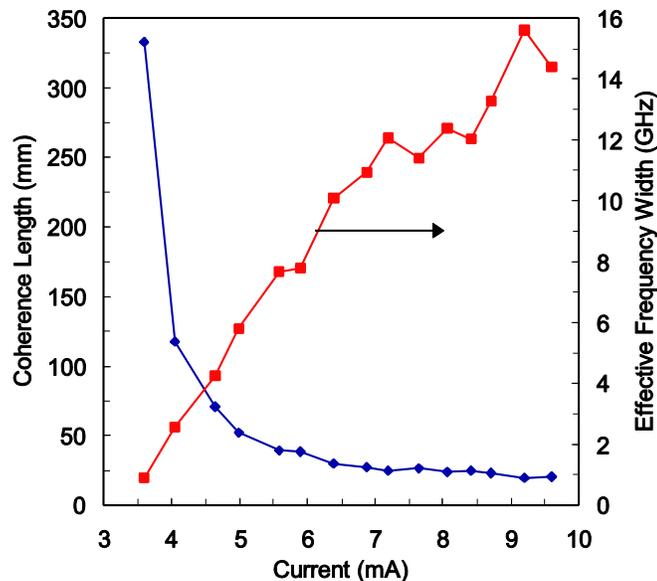
Figure 6 Coherence length and effective frequency width of a VCSEL.
