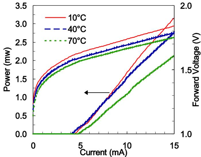
Figure 2. Typical LIV curves for 10, 40 and 70C.
