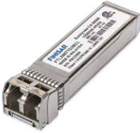
Finisar's Small-Form Factor Pluggable (SFP) transceivers provide tremendous flexibility for industrial applications. Common equipment can be designed with generic SFP ports and later the optimal transceiver can be installed for the application. This reduces R&D investments and streamlines operations.
