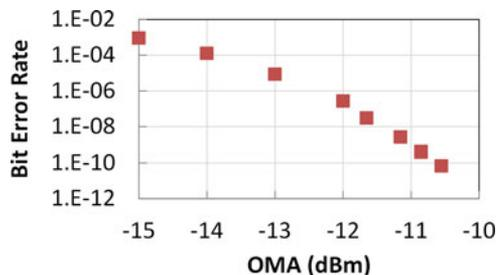
Fig. 6. Typical receiver BER sensitivity measured in the optical transceiver without FEC.
