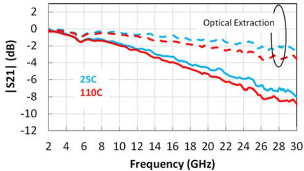
Fig. 4. Measured  $|S_{21}|$  (solid) and extracted optical response (dashed) responses for the 25 Gb/s photodiode at 25 C (blue) and 110C (red). The total capacitance is 0.115 pF. The bias voltage is 2.05 V.
