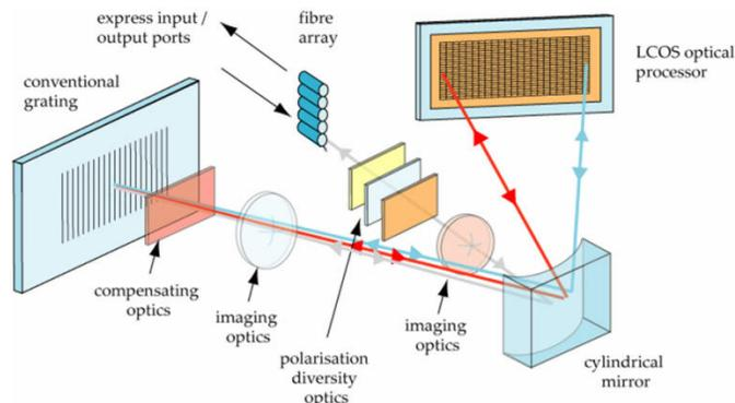
Figure 1: Simplified schematic layout of the WaveShaper 4000S.
