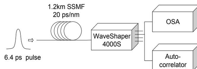
Figure 2: Experimental setup for proof of principle demonstration
