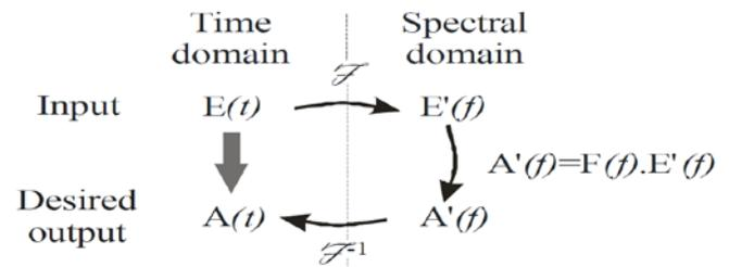
Figure 2: Diagrammatic representation of Fourier-domain pulse shaping.
